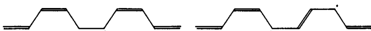
Figure 13. Topological representations of a polaron in c-PA . In contrast to the case of a soliton, the amplitude of the defect is free to vary instead of being fixed by the boundary conditions, and this is illustrated here. The right-hand diagram shows how a polaron may, in one limit, be considered as a bound soliton pair, as the chain changes from cis-transoid to trans-cisoid and back again. There are two localised electronic states; the defect will be stable if at least one is unoccupied or doubly occupied.
